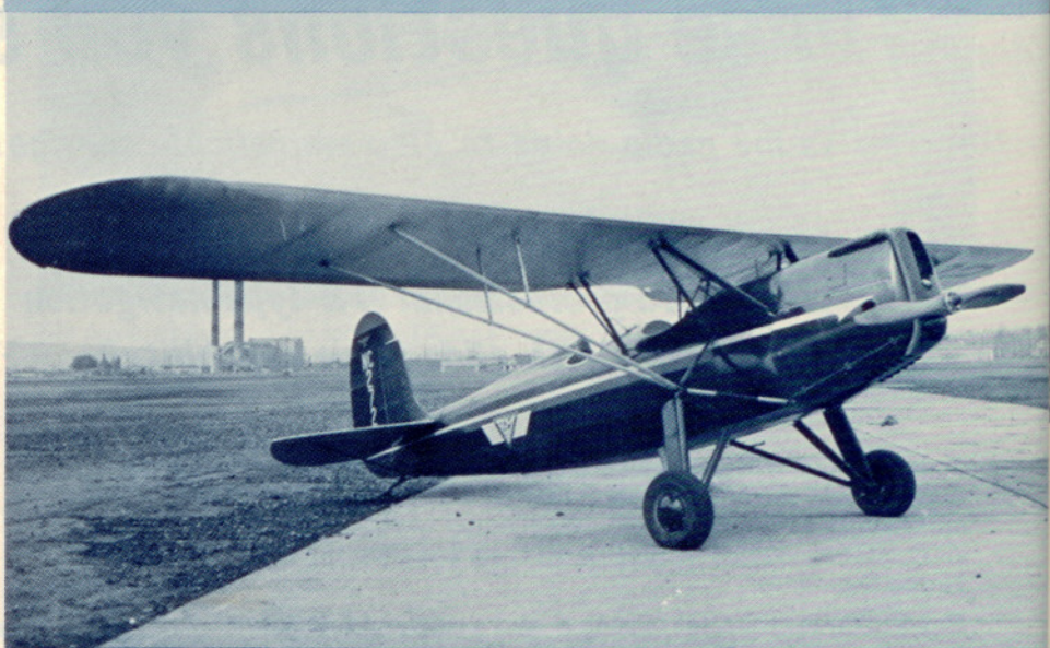
Fairchild 22C-7D, with upright four-cylinder, air-cooled Wright "Gypsy" engine Photos by the author
